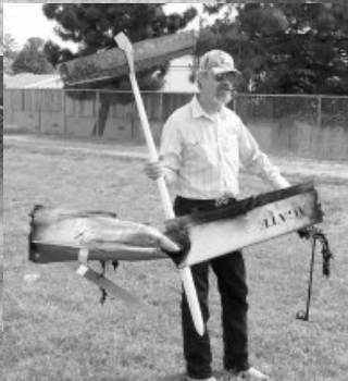
Left and Above:- These small pictures cannot do justice to the carnage caused by a carbon plane hitting high tension cables. Its a mess. The stick displayed on the left is the fuse that blew. The fuse and stabs are salvagable.
